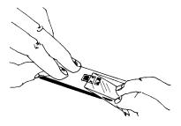
The gage and terminal strip are now solidly bonded in place. It is not necessary to remove the tape immediately after gage installation. The tape will offer mechanical protection for the grid surface and may be left in place until it is removed for gage wiring. To remove the tape, pull it back directly over itself, peeling it slowly and steadily off the surface. This technique will prevent possible lifting of the foil on open-faced gages or other damage to the installation.
