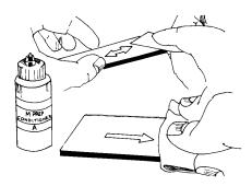
Preliminary dry abrading with 220- or 320-grit siliconcarbide paper is generally required if there is any surface scale or oxide. Final abrading is done by using 320-grit silicon-carbide paper on surfaces thoroughly wetted with M-Prep Conditioner A; this is followed by wiping dry with a gauze sponge. Repeat this wet abrading process with 400-grit silicon-carbide paper, then dry by slowly wiping through with a gauze sponge.
