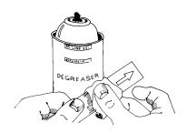
Thoroughly degrease the gaging area with solvent, such as CSM Degreaser or GC-6 Isopropyl Alcohol. The former is preferred, but there are some materials (e.g., titanium and many plastics) that react with strong solvents. In these cases, GC-6 Isopropyl Alcohol should be considered. All degreasing should be done with uncontaminated solvents-thus the use of "one-way" containers, such as aerosol cans, is highly advisable.
